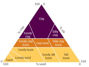
The ideal mineral soil to use for embankments generally has between 20-30% clay content. These are the soil types shown in orange in the triangle diagram above. A lower clay content may not meet the required permeability, whilst a higher one may be difficult to form into a stable embankment and could tend to shrink and crack on drying. It should however be suitable for the base.
